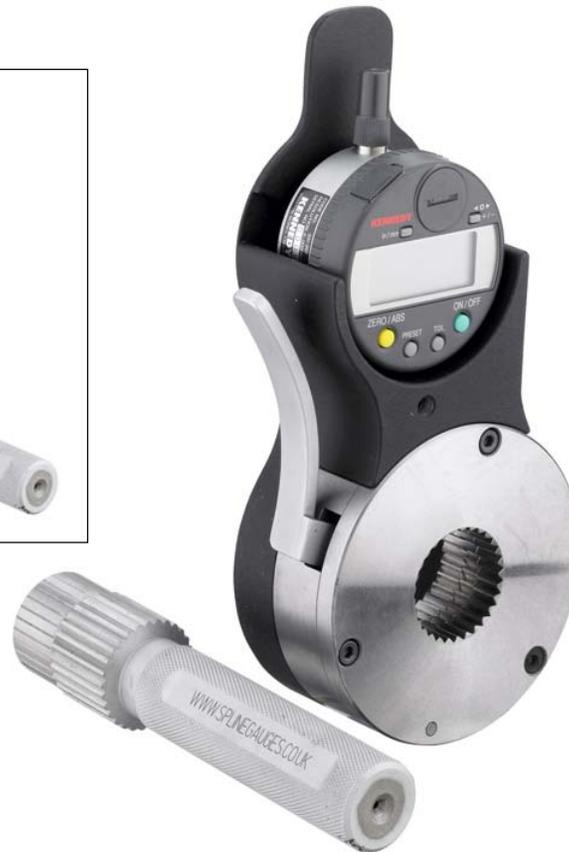
Can be supplied with analogue or digital indicators. Alternatively, a transducer port can be incorporated for SPC type analysis on PC.
