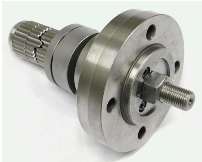
Machine face plate mounted mandrel.
