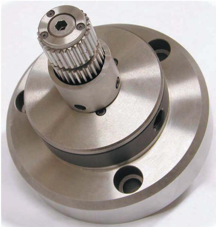
Used for the clamping of splined components. Expanding keys make this type of mandrel suitable for major diameter fitting splines.
