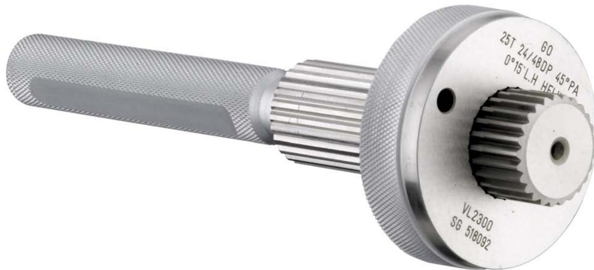
Taper tooth master plugs with fit and wear lines are used to monitor the wear of ring gauges during component manufacture. The ring gauge is ground to fit the master plug for original and replacement ring gauges.
