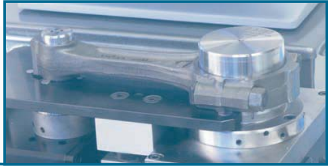
Connecting Rod Bend & Twist Gage checks parallelism and center distance between piston end and crank end bores. Inspection system includes custom gaging fixture, quad AEK air-electric converter, and Gage-Chek Readout.
