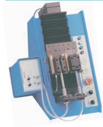
Three Spindle Inspection station checks bore size, O.D. size, I.D. to O.D. concentricity, and bore to face perpendicularity on machined bearing housing. Uses 3 quad AEK air/electric converters coupled to CWK-2 computer.
