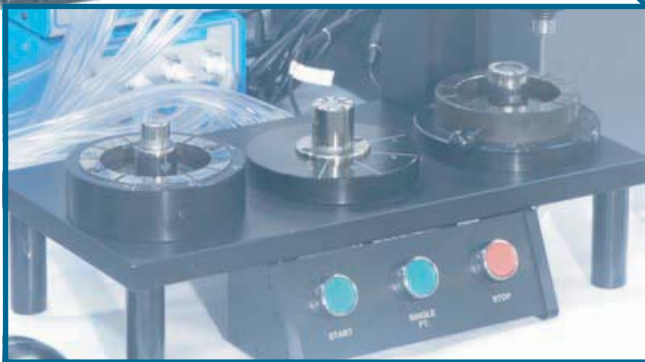
Three Spindle Inspection station checks bore size, O.D. size, I.D. to O.D. concentricity, and bore to face perpendicularity on machined bearing housing. Uses 3 quad AEK air/electric converters coupled to CWK-2 computer.
