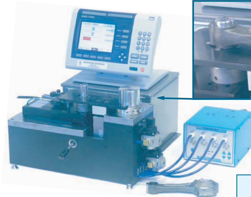
Connecting Rod Bend & Twist Gage checks parallelism and center distance between piston end and crank end bores. Inspection system includes custom gaging fixture, quad AEK air-electric converter, and Gage-Chek Readout.
