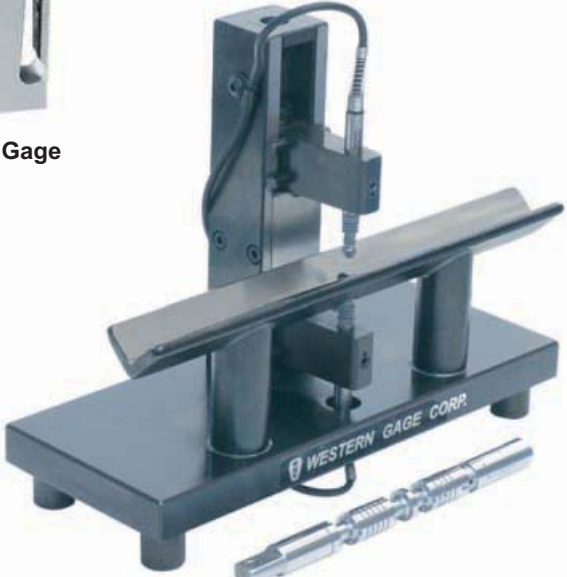
Vee Gage checks hydraulic valve spool O.D.s utilizing opposed set of LVDT Inductive Probes.
