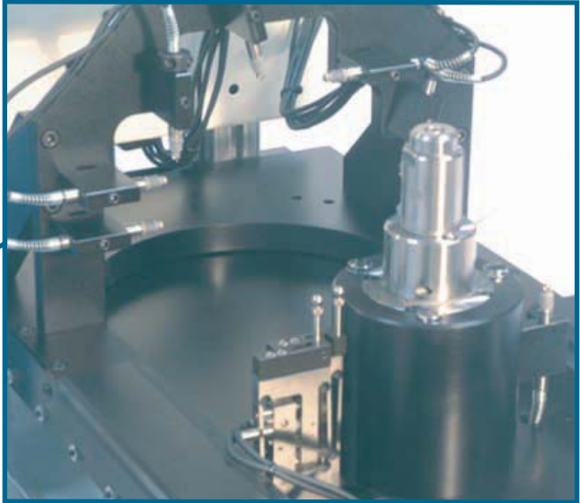
Air Spindle, LVDT Inductive probes & Flexure gages used in inspection stations for scroll compressor parts.
